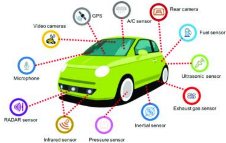
Different types of built in-vehicle sensors.
