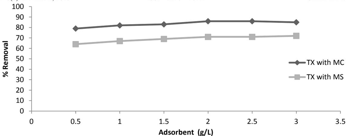
**Fig. 2: Effect of Adsorbent Dose for the Removal of Colour from Textile Effluent with Maize Cob and Mahogany Shell**
