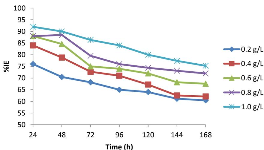
**Fig. 2:** Effect of Immersion Time (hrs) on Inhibition Efficiency of *N. imperialis* Seeds Extract for the Corrosion of Mild Steel in 1.0 M HCl.
