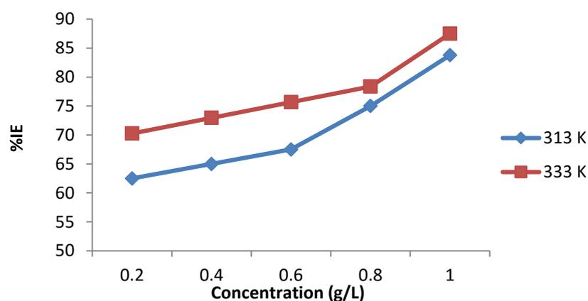
**Fig. 4:** Effect of Concentrations of *N. imperialis* Seeds Extract on Inhibition Efficiency for the Corrosion of Mild Steel in 1.0 M HCl at 313 and 333 K.
