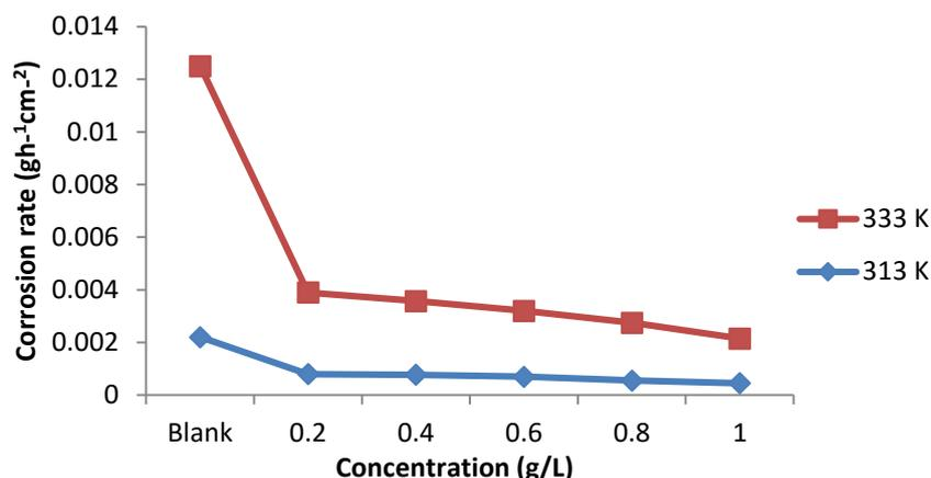
**Fig. 3:** Effect of Concentrations of *N. imperialis* Seeds Extract on the Corrosion Rate of Mild Steel in 1.0M HCl at 313 and 333 K.
