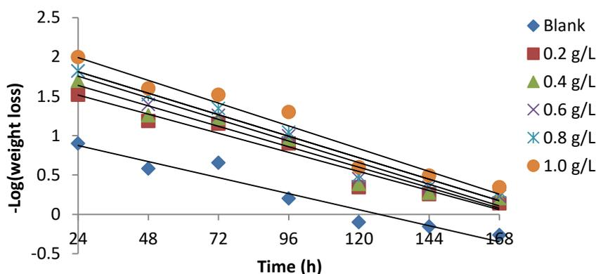
**Fig. 5:** Plots of  $-\text{Log}(\text{Weight Loss})$  Versus Time for the Corrosion of Mild Steel in the Absence and Presence of *N. imperialis* Seeds Extract in 1.0 M HCl.
