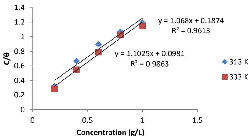
**Fig. 6:** Langmuir Isotherms for the Adsorption *N. imperialis* Seeds Extract on Mild Steel Surface in 1.0 M HCl at 313 and 333 K.
