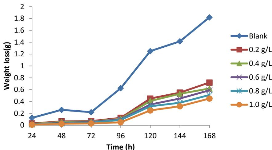
**Fig. 1:** Effect of Immersion Time (hrs) on Weight Loss (g) of Mild Steel in 1.0 M HCl in the Absence and Presence of *N. imperialis* Seeds Extract.
