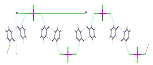
**Figure 3:** A hydrogen-bonded ribbon in [H<sub>2</sub>pymo]<sub>2</sub>[ZnCl<sub>4</sub>].
