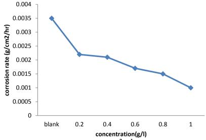
Fig 1: Variation of Corrosion Rate (g cm<sup>-2</sup> h<sup>-1</sup>) of Aluminum against Various Concentrations of *Cissus populnea* Stem Extract in 0.5 M HCl at 303 K.
