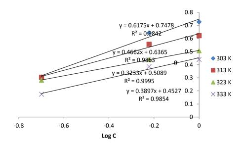
Fig 9: Temkin Isotherm for the Adsorption of *Cissus populnea* Stem Extract on Aluminum Surface in 0.5 M HCl at 303 – 333 K.
