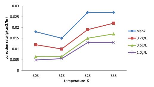
Fig 5: Variation of Corrosion Rate of Aluminum Against Temperature (303 – 333 K) in the Absence and Presence Different Concentrations of *Cissus populnea* Stem Extract in 0.5 M HCl.
