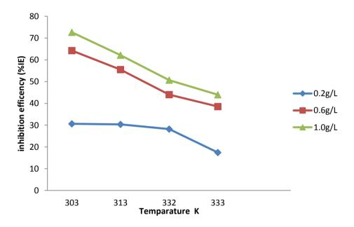
Fig 6: Variation of Inhibition Temperature (%IE) Against Temperature for the Corrosion of Aluminum in 0.5 M HCl in the presence and absence of Cissus populnea stem extract.
