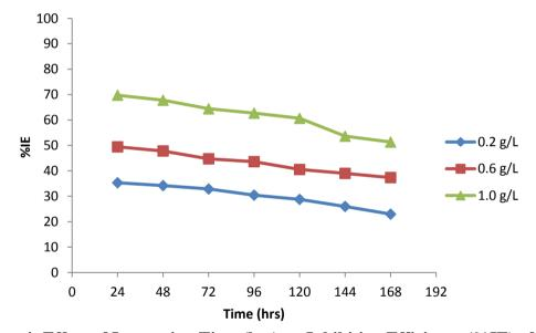
Figure 4: Effect of Immersion Time (hrs) on Inhibition Efficiency (%IE) of *Cissus* populnea Stem Extract on the Dissolution of Aluminum in 0.5 M HCl at 303 K.
