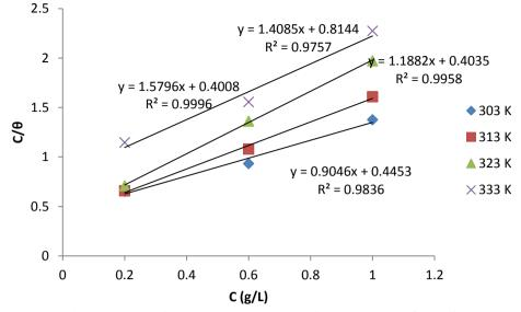
Fig 8: Langmuir Isotherm for the Adsorption of *Cissus populnea* Stem Extract on Aluminum Surface in 0.5 M HCl at 303 – 333 K.
