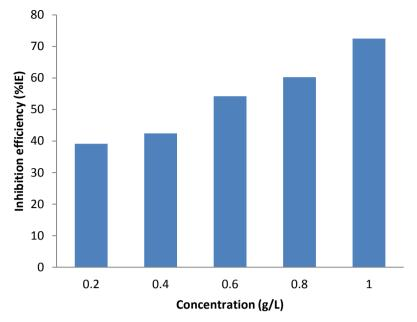
Fig 2: Variation of Inhibition Efficiency (%IE) against Various Concentrations of *Cissus populnea* Stem Extract for Aluminum Corrosion in 0.5 M at 303 K.
