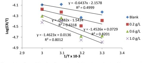
Fig 10: Transition State Plots for Corrosion of Aluminum in the Absence and Presence of Different Concentrations of *Cissus populnea* Stem Extract.
