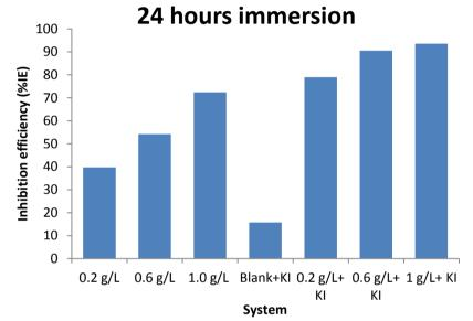
Fig 7: Effect of the Addition of 0.05 M KI on the Corrosion of Aluminum in 0.5 M HCl at 303 K.
