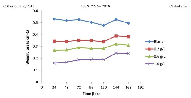
Fig 3: Effect of Immersion Time (hrs) on Corrosion Rate of Aluminum in 0.5 M HCl in the Absence and Presence of *Cissus populnea* Stem Extract at 303 K.
