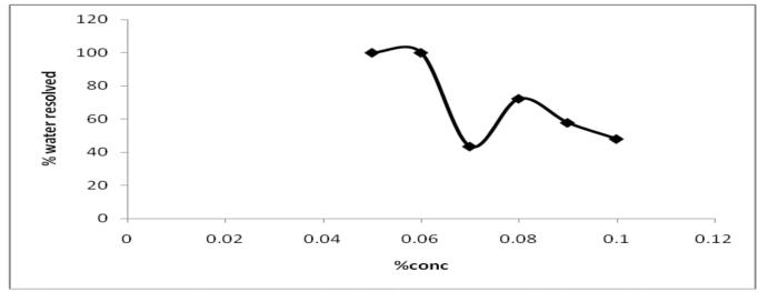
Fig.2: Percent water resolved in an emulsion as a function of asphaltene concentration in model oil after 2880 minutes
