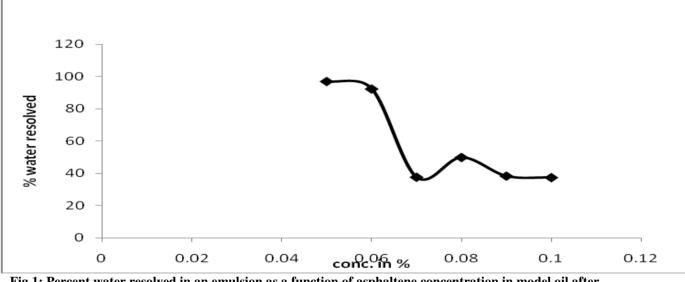
Fig.1: Percent water resolved in an emulsion as a function of asphaltene concentration in model oil after 1440 minutes.
