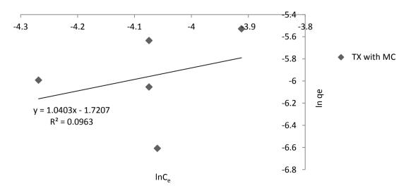
Fig. 4; Freundlich Isotherm for Colour Adsorption onto Maize Cob
