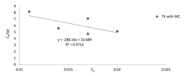
Fig. 6: Langmuir Isotherm for Colour Adsorption onto Maize Cob
