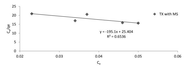
Fig. 7: Langmuir Isotherm for Colour Adsorption onto Mahogany Shell
