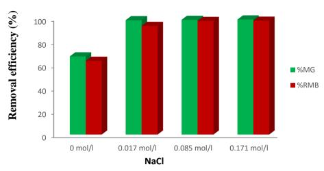
**Fig. 3:** Effect of Salt on the Adsorption of RdB and MG onto Bentonite at the Initial dye concentration of 30 mg/l.
