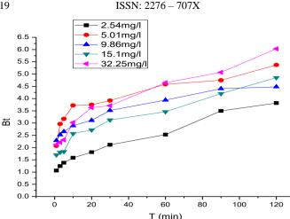
FIG 4: Boyd kinetic plot for the sorption of RdB onto Bentonite at different initial concentrations.
