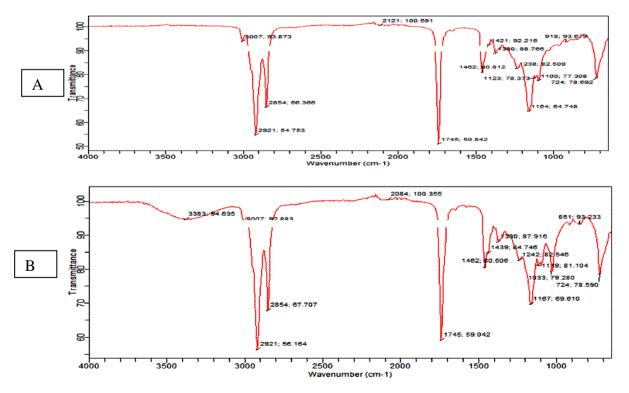
Figure 2: FTIR spectrum of oil (A) and *B.aegyptiaca* biodiesel/FAME (B)
