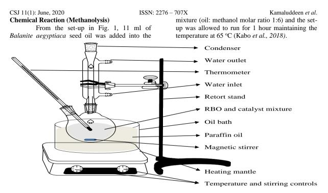
Figure 1: Experimental Set-up for Methanolysis Reaction
