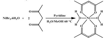
Scheme 2: Synthesis of [Ni(acac)<sub>2</sub>2H<sub>2</sub>O]
