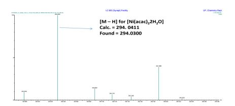
Fig. 5: HRMS spectra of [Ni(acac)<sub>2</sub>.2H<sub>2</sub>O]
