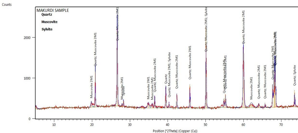
**Figure 6: Diffractogram for Makurdi Clay-Rich Soils**
