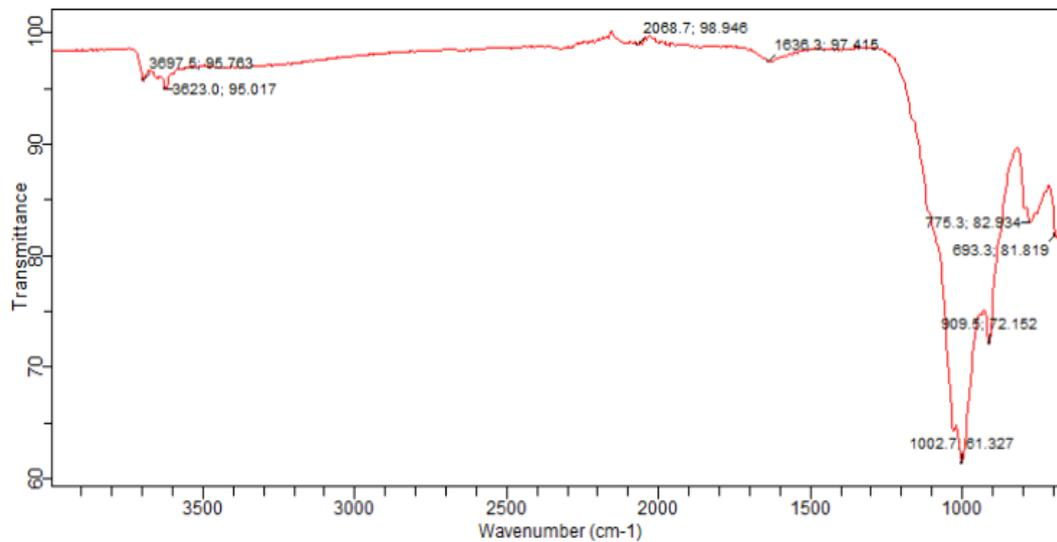
Figure 9: Fourier Transform Infra-red Spectrum of Clay-Rich Soils from Makurdi
