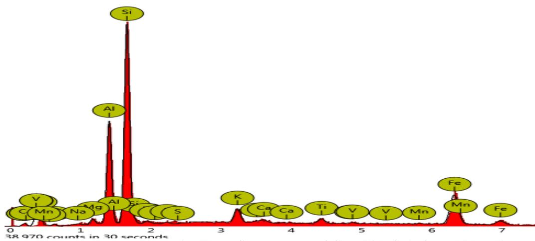
Figure 3: Energy Dispersive X-ray Spectroscopy of Clay-Rich Soils from Makurdi
