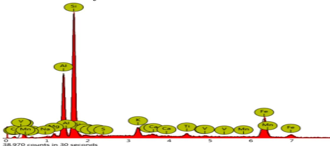
**Figure 2: Energy Dispersive X-ray Spectroscopy of Clay-Rich Soils from Angbaaye**
