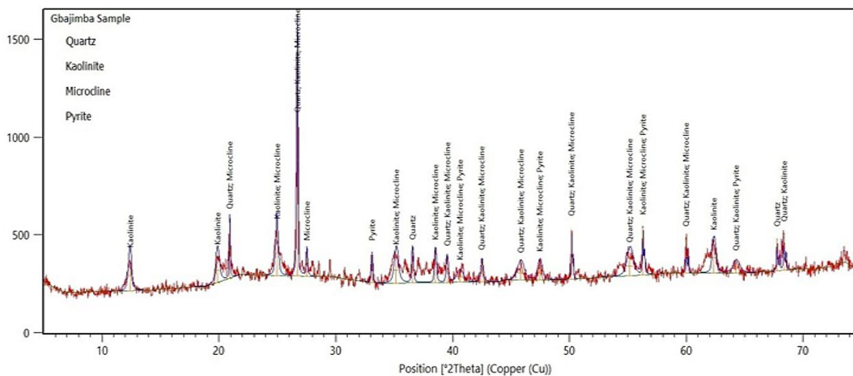
**Figure 5: Diffractogram for Gbajimba Clay-Rich Soils**
