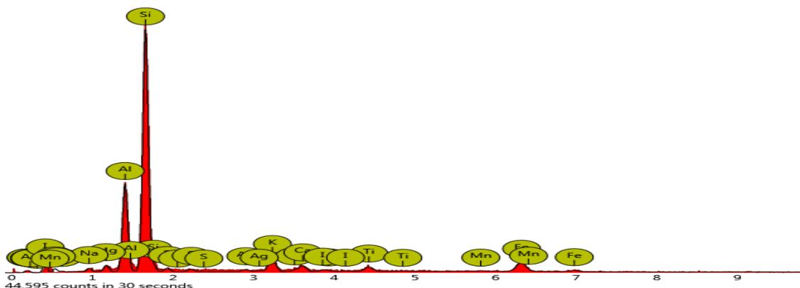
**Figure 1: Energy Dispersive X-ray Spectroscopy of Clay-Rich Soils from Gbajimba**
