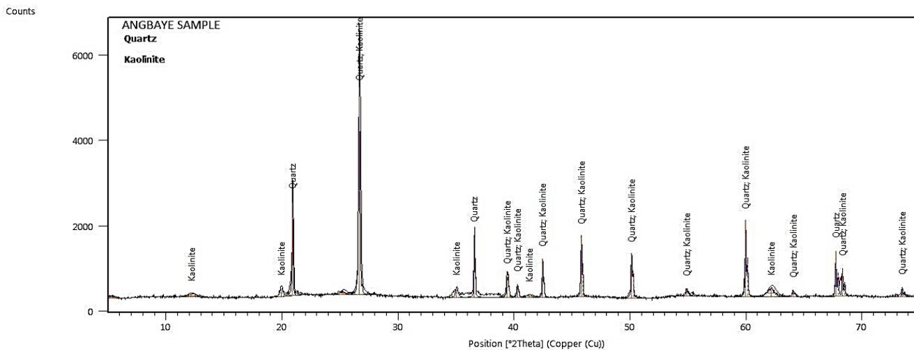
**Figure 4: Diffractogram for Angbaaye Clay-Rich Soils**
