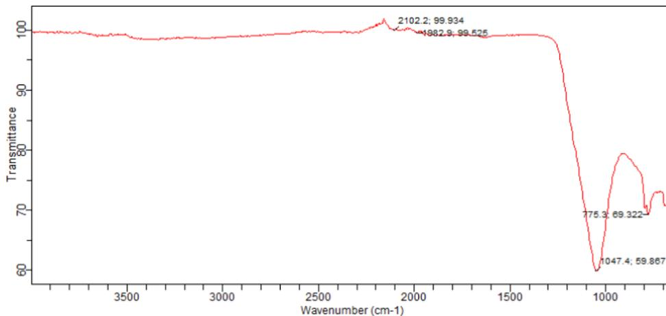
Figure 7: Fourier Transform Infra-red Spectrum of Clay-Rich Soil from Gbajimba
