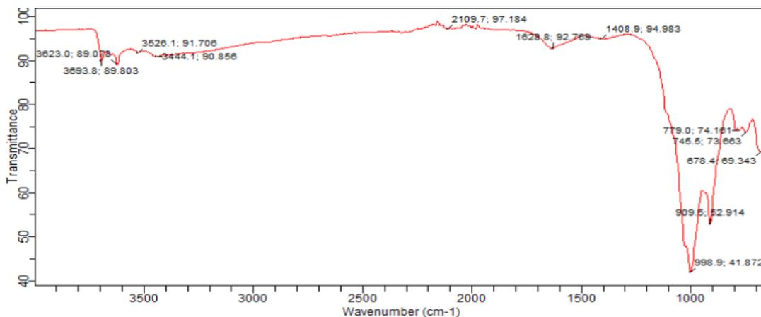
Figure 8: Fourier Transform Infra-red Spectrum of Clay-Rich Soil from Angbaaye
