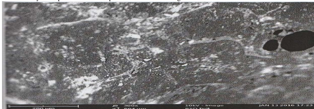
**Figure 7:** SEM of 75% PMMA 25% PVC blend before burial
