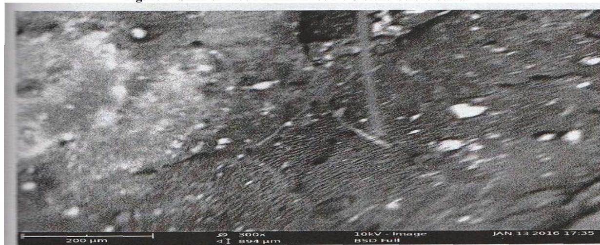
**Figure 8:** SEM of 75%PMMA/25%PVC blend after burial
