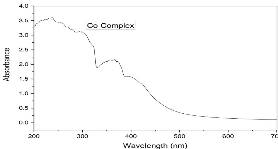
**Figure 6: Uv-Vis Spectra of Co-Complex**
