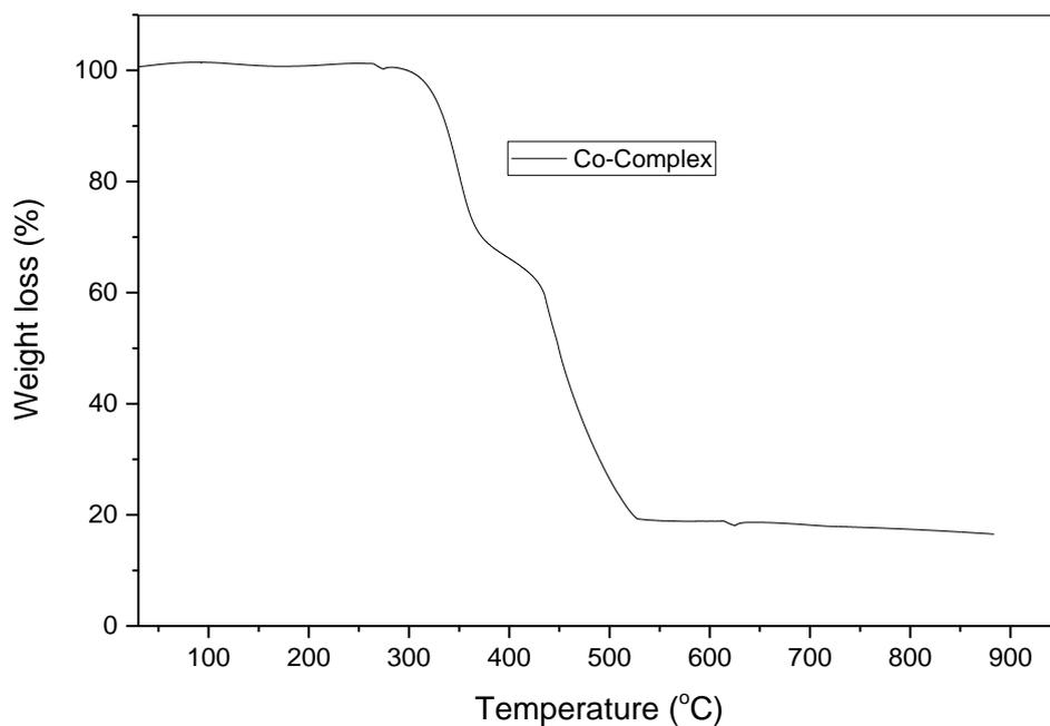
**Figure 8: Co-Complex TGA Spectra**
