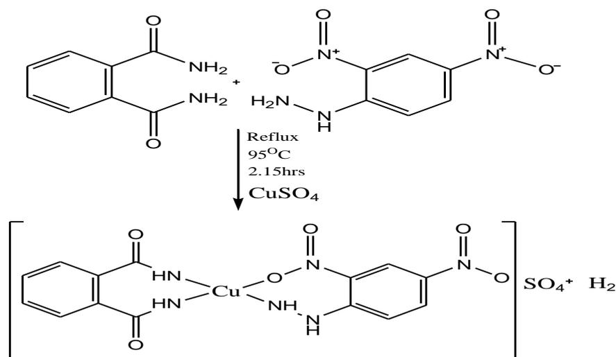
Fig. 1: Synthetic route of the reaction of Cu-Complex
