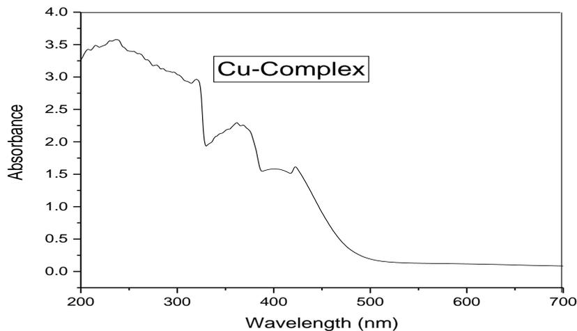
**Figure 5: Uv-Vis Spectra of Cu-Complex**
