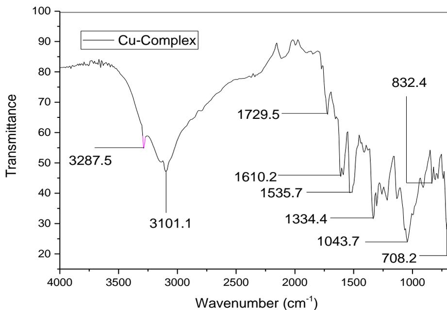
**Figure 3: Cu-Complex IR-Spectra**
