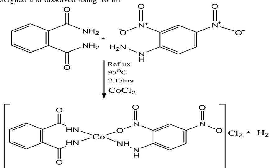
Fig. 2: Synthetic route of the reaction of Co-Complex
