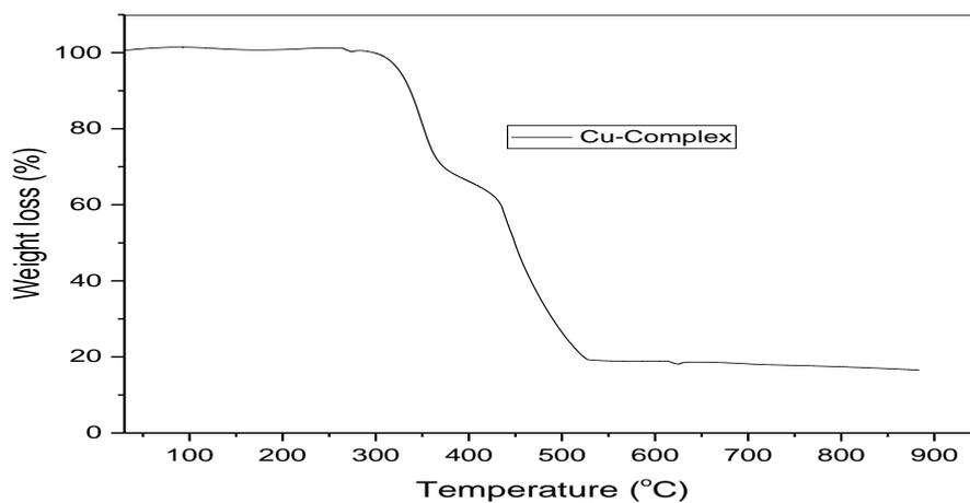
**Figure 7: Cu-Complex TGA Spectra**
