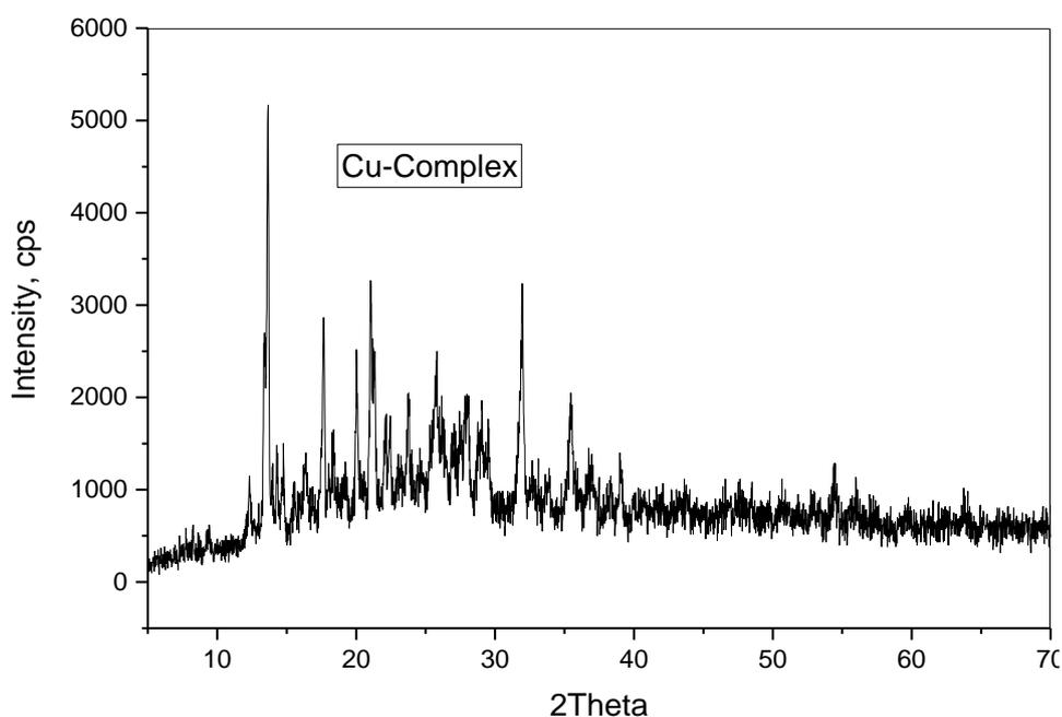
**Figure 9: Cu-Complex XRD Spectra**
