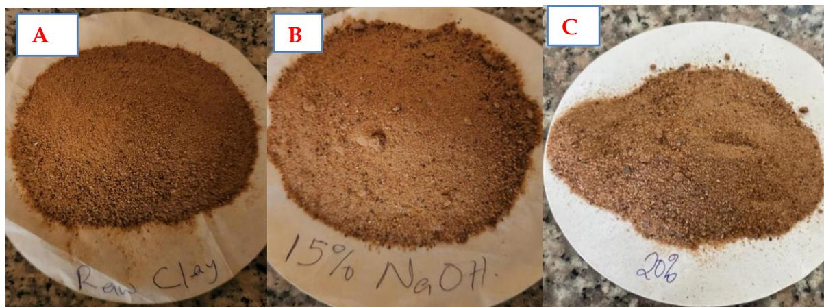
**Fig. 1: (A) Raw Clay (B) 15% NaOH Modified Clay (C) 20% NaOH Modified Clay**
