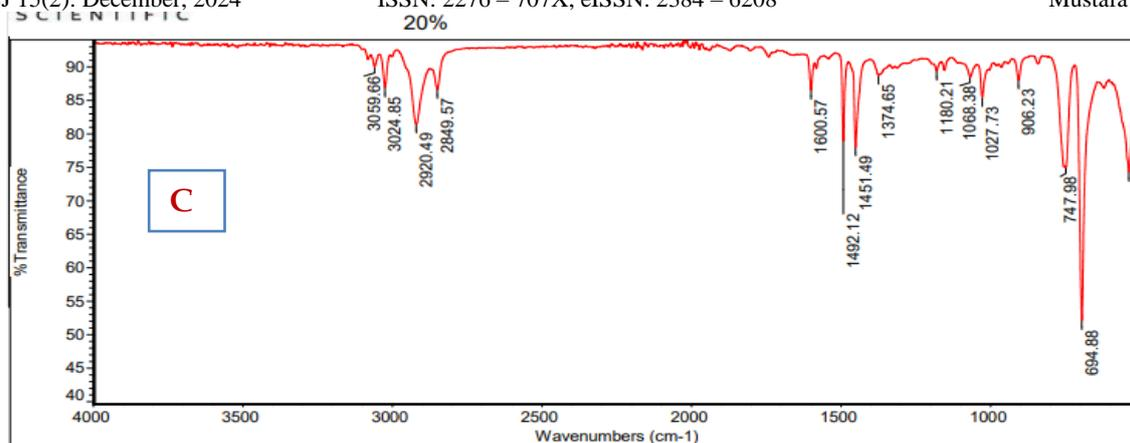
**Fig. 3: FTIR SPECTRA (A) Raw Clay (B) 15% NaOH modified Clay (C) 20% NaOH modified Clay**
