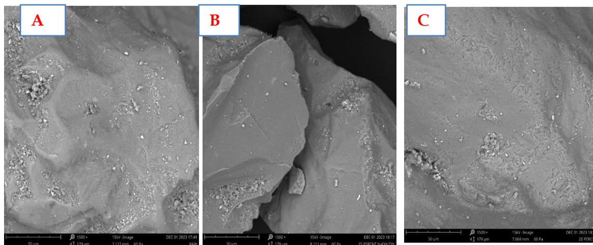
**Fig. 2: SEM Micrographs (A) Raw Clay (B) 15% NaOH Modified Clay (C) 20% NaOH Modified Clay at 1500 Magnification**
