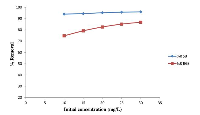
Fig. 4: Variation in % Removal with Initial Dye Loading Concentration
