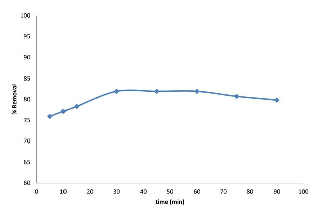
Fig. 2a: Estimation of Adsorption Equilibrium Time using Sugarcane Bagasse
