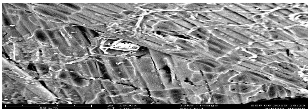
**Fig. 12: SEM Image of *Albizia lebeck* Shells after Adsorption of Basic Malachite Green**
