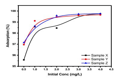
**Figure 2:** Effect of initial concentration on adsorption of Zn ions by chemically modified sample X, Y and Z at room temperature and pH 4
