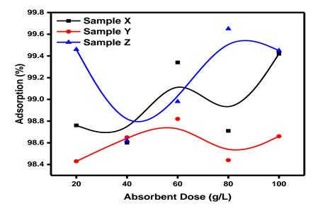
**Figure 8:** Effect of adsorbent dose on adsorption of Zn ions by chemically modified sample X, Y and Z with initial concentration 2 mg/L at room temperature and pH 4
