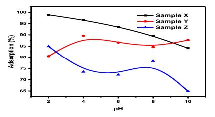
**Figure 5:** Effect of pH on adsorption of Pb (II) ions by chemically modified sample X, Y and Z with initial concentration 10 mg/L at room temperature and pH 4
