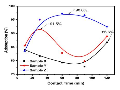
**Figure 3:** Effect of contact time on adsorption of Pb (II) ions by chemically modified sample X, Y and Z with initial concentration 10 mg/L, at room temperature and pH 4
