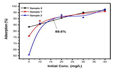
**Figure 1:** Effect of initial concentrations on adsorption of Pb (II) ions by chemically modified sample X, Y and Z at room temperature and pH 4
