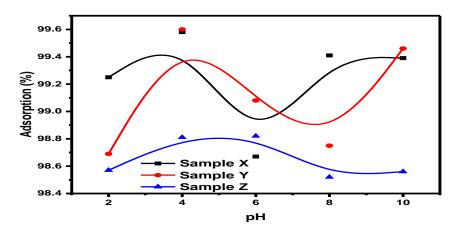
**Figure 6:** Effect of pH on adsorption of Zn ions by chemically modified sample X, Y and Z with initial concentration 2 mg/L at room temperature and pH 4
