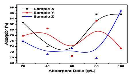
**Figure 7:** Effect of adsorbent dose on adsorption of Pb (II) ions by chemically modified samples X, Y, Z with initial concentration 10 mg/L at room temperature and pH 4
