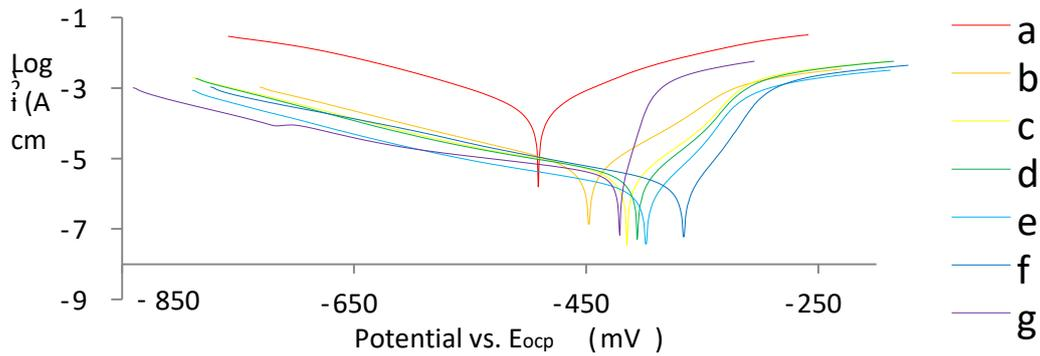
**Figure 5:** Polarization curves of stainless steel in 1 M H<sub>2</sub>SO<sub>4</sub> in the presence of different concentrations of both extracts with KI: (a) blank; (b) 0.3 g/L SCM (c) 0.5 g/L SCM (d) 0.3 g/L PCM (e) 0.5 g/L PCM (f) 0.7 g/L PCM (g) 0.7 g/L SCM
