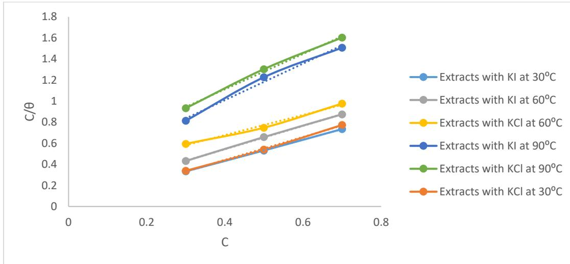
**Figure 7:** Langmuir isotherm for peel extract of stainless steel corrosion in 1M H<sub>2</sub>SO<sub>4</sub>. The plot of log CR versus 1/T produces straight lines as shown in Figures 8 and 9 which indicates the Arrhenius adsorption isotherm.
