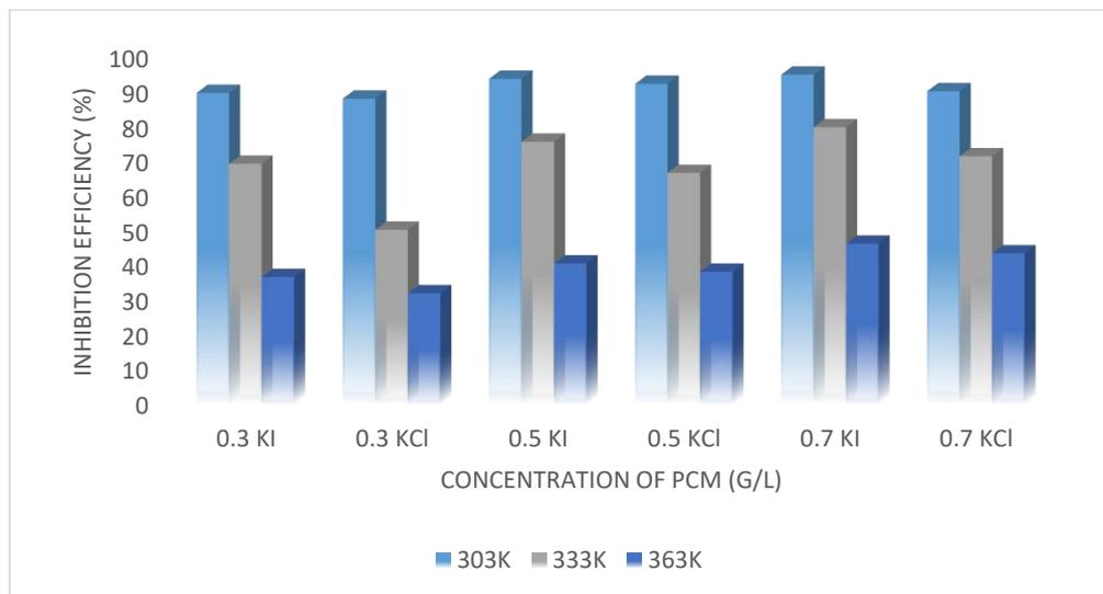
Figure 4: Inhibition efficiency of Peel extract of *C.maxima*
