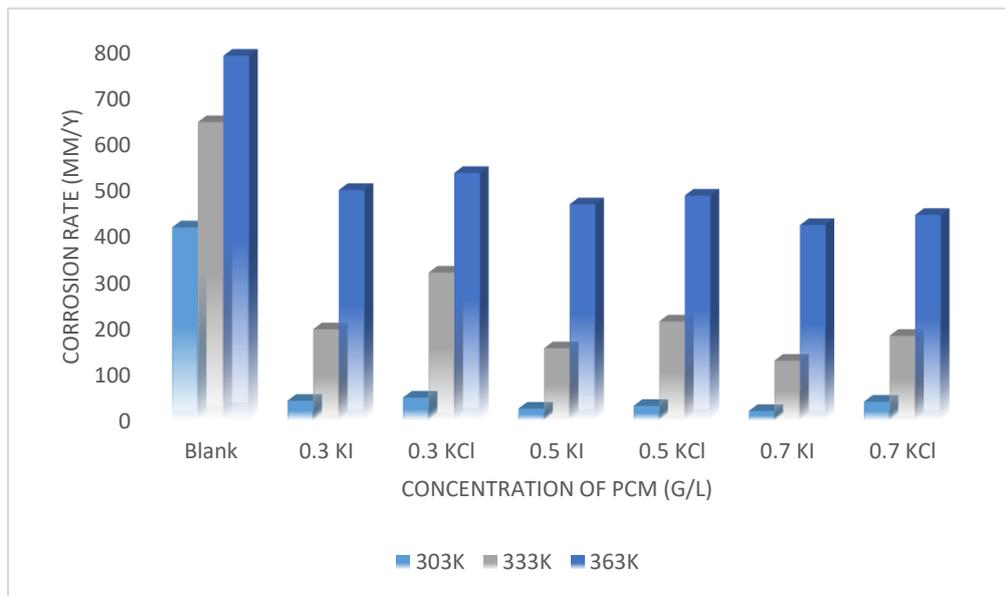
Figures 3: Corrosion rate of Peel extract of *C. maxima*
