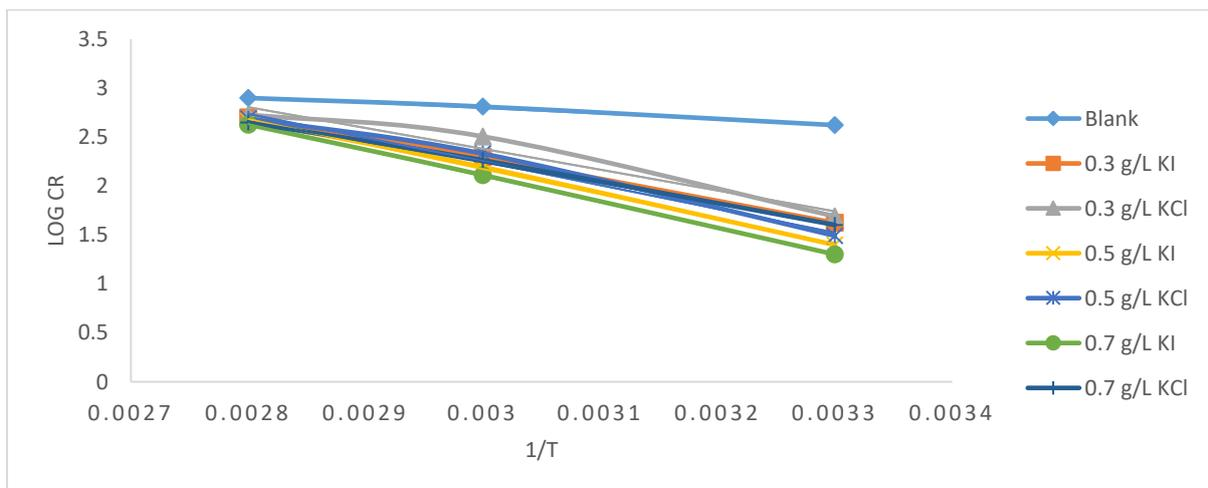
**Figure 9:** Plot of log CR versus 1/T for Peel extract
