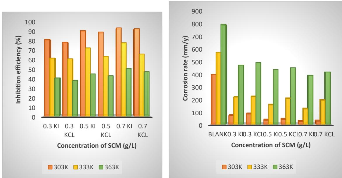
Figures 1 and 2: Corrosion rate and inhibition efficiency of Seed extract of *C. maxima*
