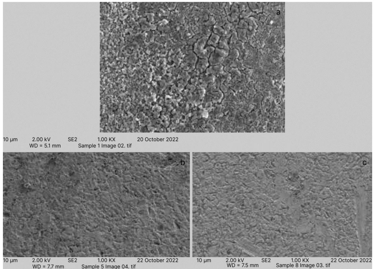
**Plate 1:** SEM images of stainless steels after corrosion in 1 M H<sub>2</sub>SO<sub>4</sub> and with both extracts at 303 K (a) Blank (b) 0.7 g/L SCM (c) 0.7 g/L PCM
