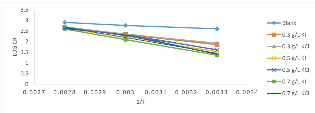
**Figure 8:** Plot of log CR versus 1/T for Seed extract
