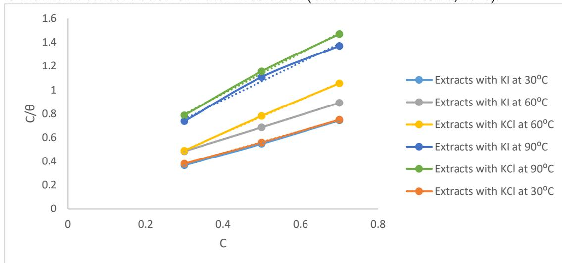
**Figure 6:** Langmuir isotherm for seed extract of stainless steel corrosion in 1M H<sub>2</sub>SO<sub>4</sub>
