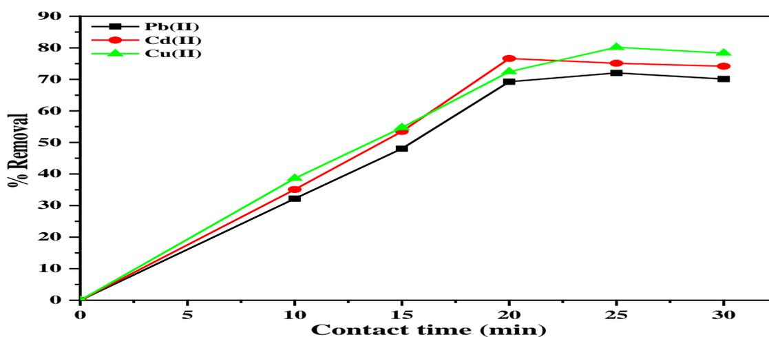
Figure 5: Effect of contact time on the removal of heavy metal ions
