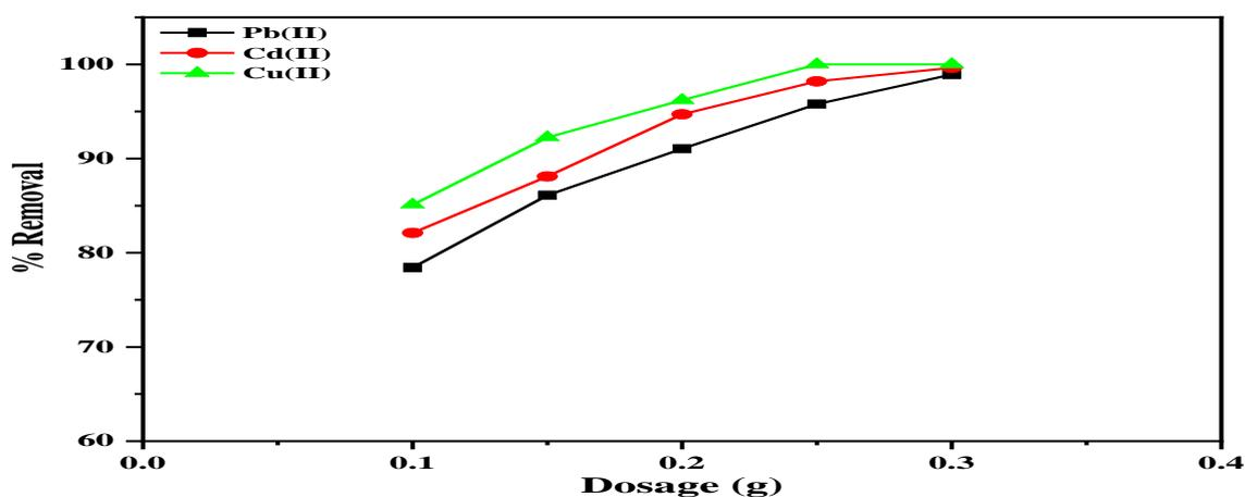
Figure 6: Effect of dosage on the removal of heavy metal ions
