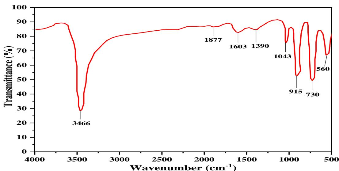
Figure 4: FTIR spectrum of Fe<sub>3</sub>O<sub>4</sub>/ZnO nanocomposites
