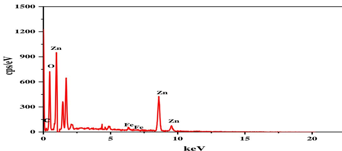
Figure 3: EDX spectrum of Fe<sub>3</sub>O<sub>4</sub>/ZnO nanocomposites
