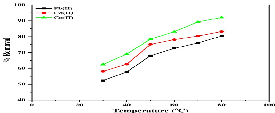
Figure 7: Effect of temperature on the removal of heavy metal ions
