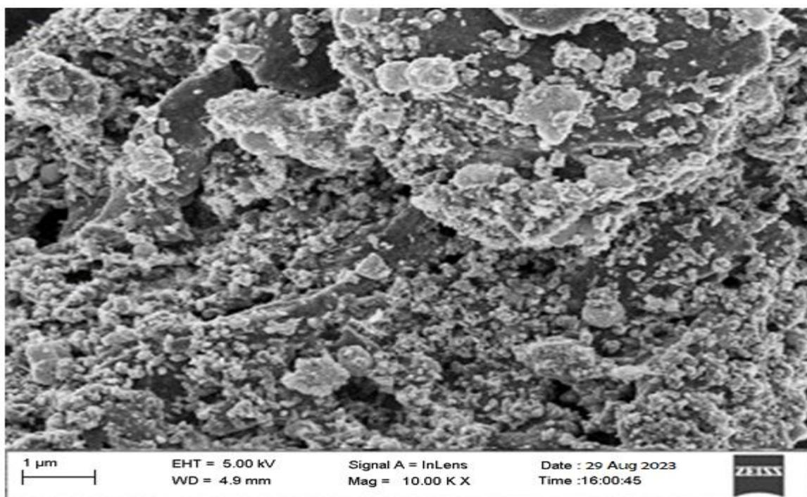
Figure 2: SEM image of Fe<sub>3</sub>O<sub>4</sub>/ZnO nanocomposites
