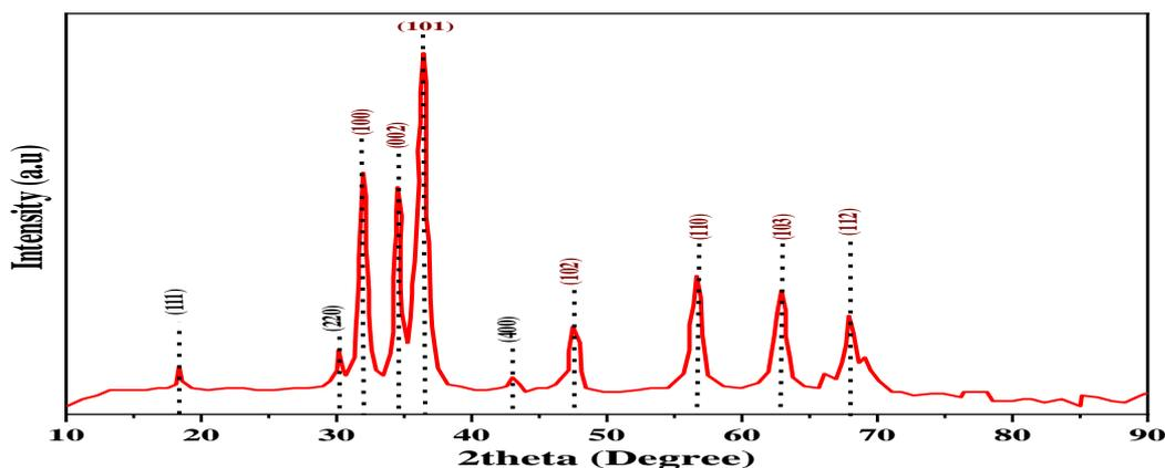
Figure 1: XRD result of Fe<sub>3</sub>O<sub>4</sub>/ZnO nanocomposites
