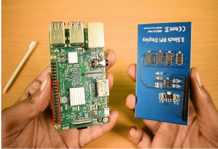
Figure 8: Installing LCD Display on Raspberry Pi
