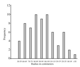
Radii of curvature of locally available femoral nails: The radii of curvature of the femoral nails ranged between 127cm and 200cm. The SIGN Nail, which is widely used now, however is a straight nail, but with a 90 proximal bend and a 1.50 distal bend to aid in insertion. The rest of the femoral nails had their radii as shown in Table 1.
