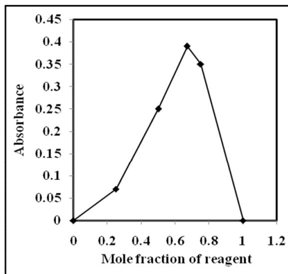
Figure 4: Determination of stoichiometric ratio of drug/reagent adduct.
