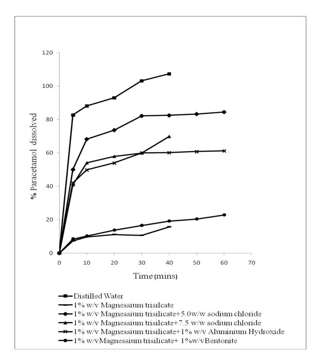
Figure 1. The effect of antacid on the dissolution profile of paracetamol from tablets in various media at  $37\pm0.5$  °C.
