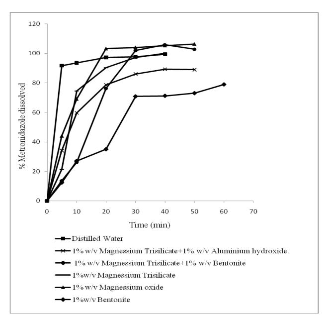
Figure 2. The effect of antacid on the dissolution profile of metronidazole from tablets in various media at  $37\pm0.5$  °C.
