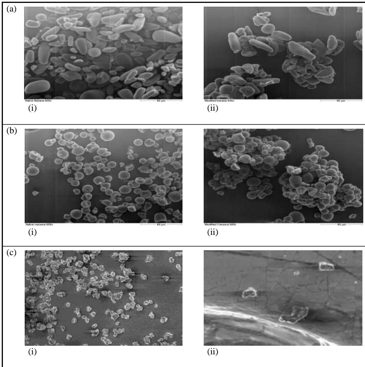
**Figure 1: Scanning electron micrographs of (a) banana, (b) cassava and (c) Chinese yam starches in the (i) native and (ii) carboxymethylated forms.**
