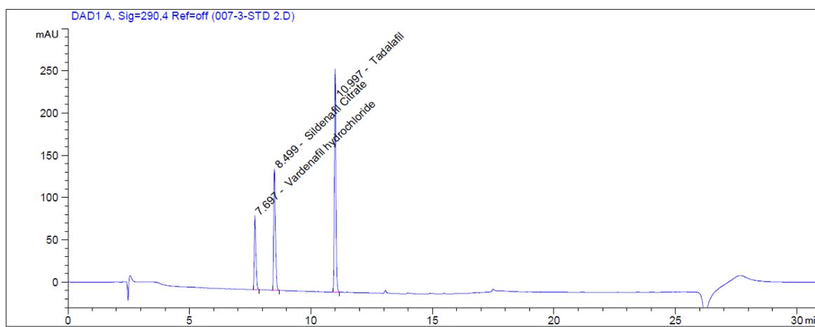
**Figure 2: HPLC chromatogram for reference standard showing chromatographic peaks at a retention times of 7.697 min, 8.499 min and 10.997 min corresponding to vardenafil hydrochloride, sildenafil citrate and tadalafil respectively.**
