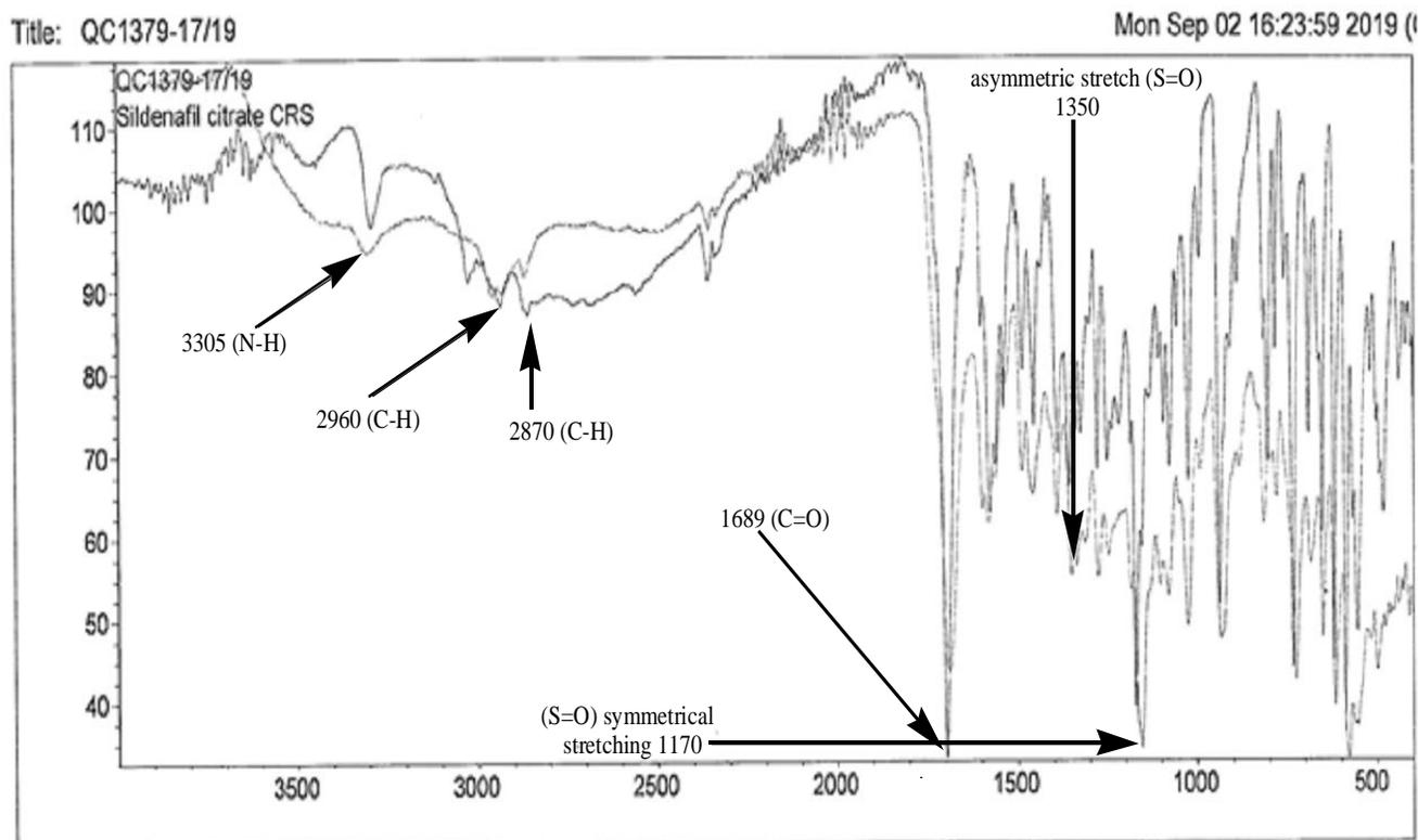
**Figure 8: Overlay FTIR spectrum of isolated compound obtained from sample QC1379-17/18 and that of sildenafil citrate reference standard.**
