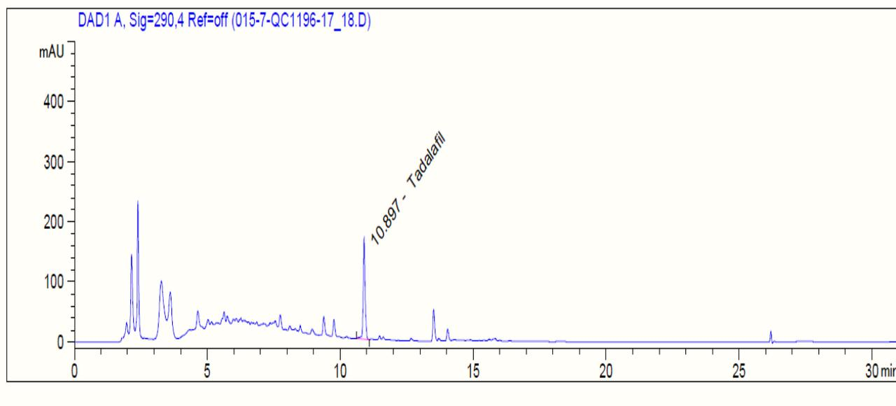
**Figure 7: HPLC chromatogram for sample QC1196-17/18 with a chromatographic peak at 10.897 min corresponding to tadalafil**
