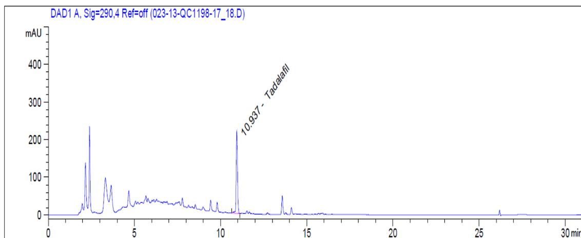
**Figure 4: HPLC chromatogram for sample QC1198-17/18 with a chromatographic peak at 10.937 min corresponding to tadalafil**
