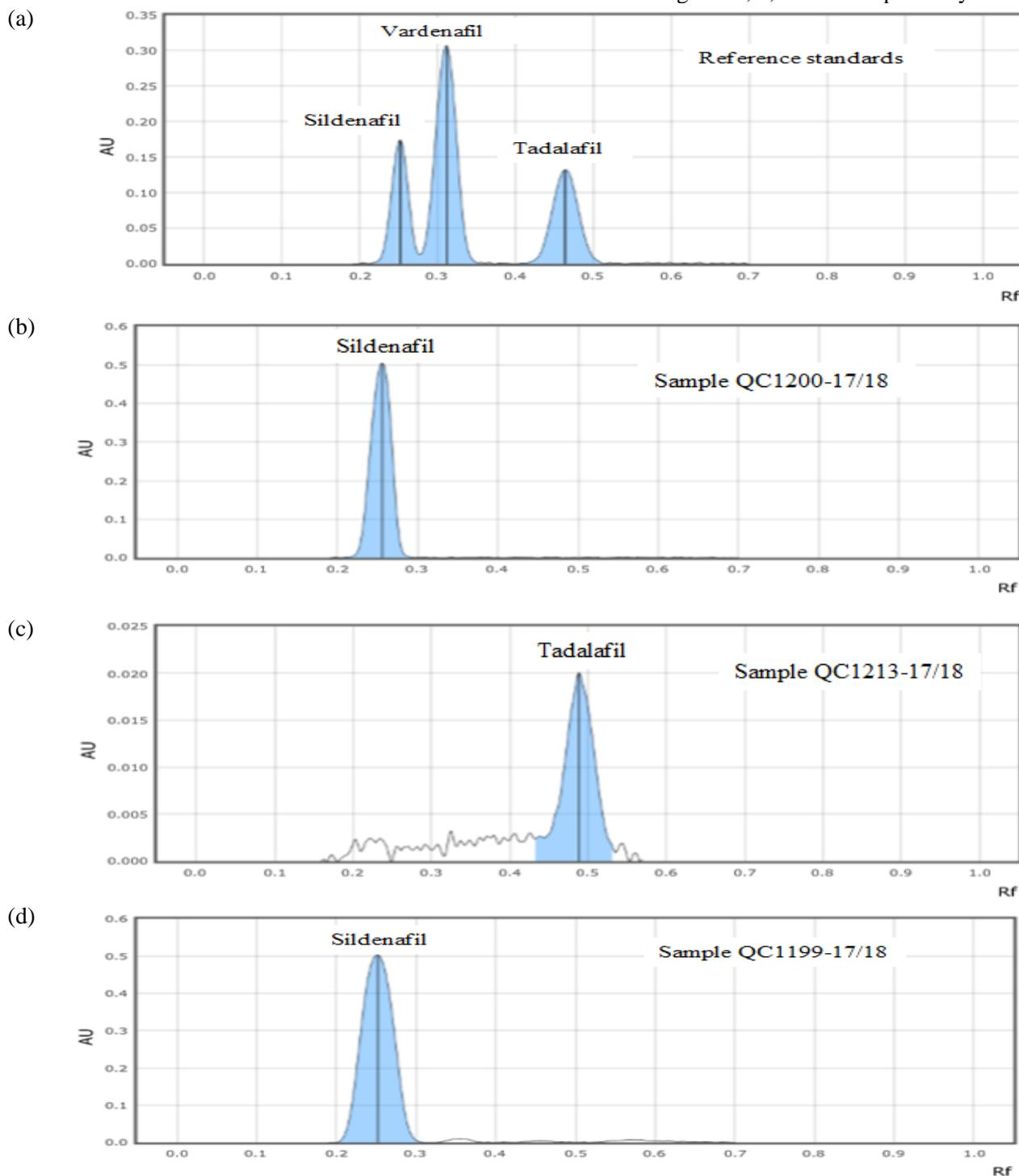
**Figure 1: HPTLC densitograms for (a) reference standard solution, (b) sample QC1200-17/18, (c) sample QC1213-18/19 and (d) sample QC1199-17/18**
