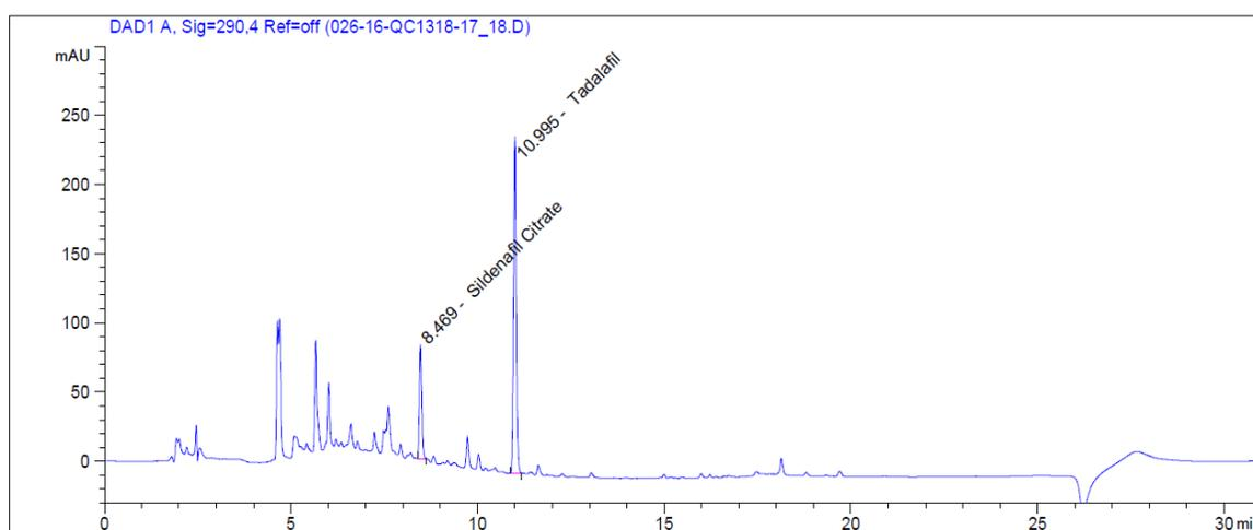
**Figure 3: HPLC chromatogram for sample QC1318-17/18 with chromatographic peaks at retention times of 8.469 min and 10.995 min corresponding to sildenafil and tadalafil**
