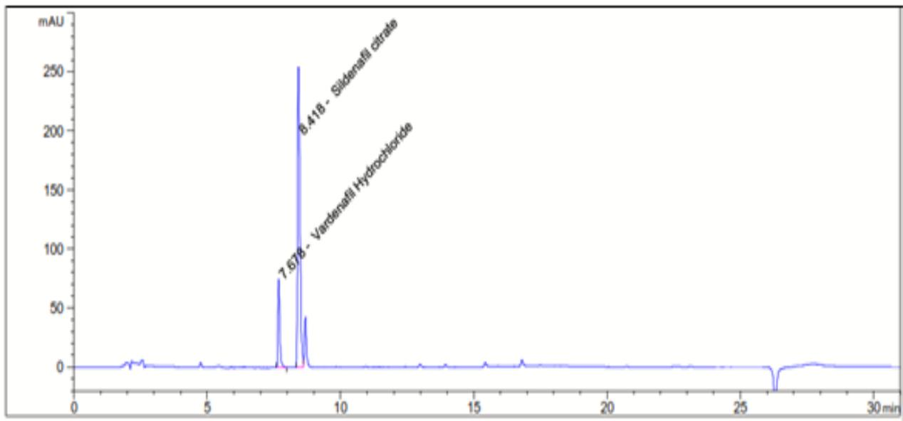
**Figure 6: HPLC chromatogram for sample QC1309-17/18 with a chromatographic peak at 7.578 min and 8.418 min corresponding to vardenafil hydrochloride and sildenafil citrate**
