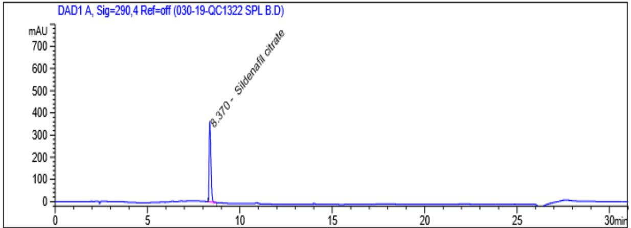
**Figure 5: HPLC chromatogram for sample QC1322-17/18 with a chromatographic peak at 8.370 min corresponding to sildenafil citrate**
