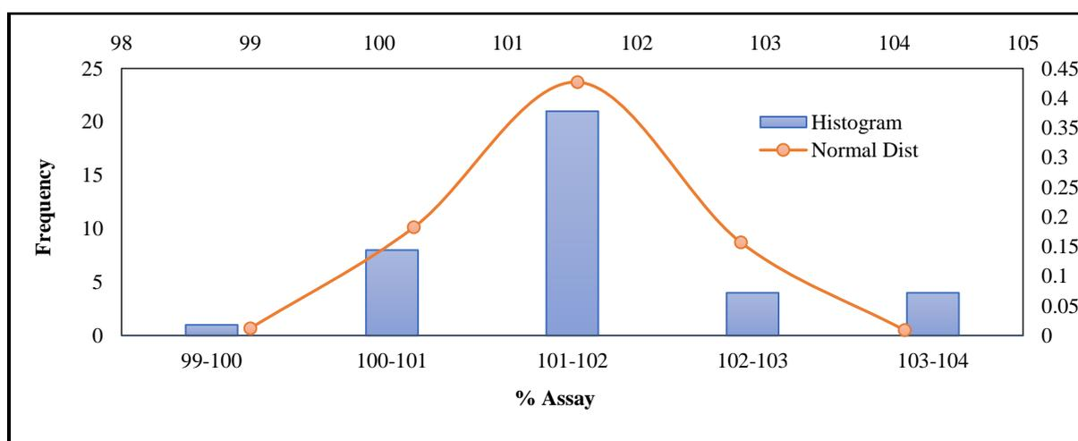
**Figure 3: Assay results for ibuprofen coated tablets represented with a histogram and normal distribution overlay.**
