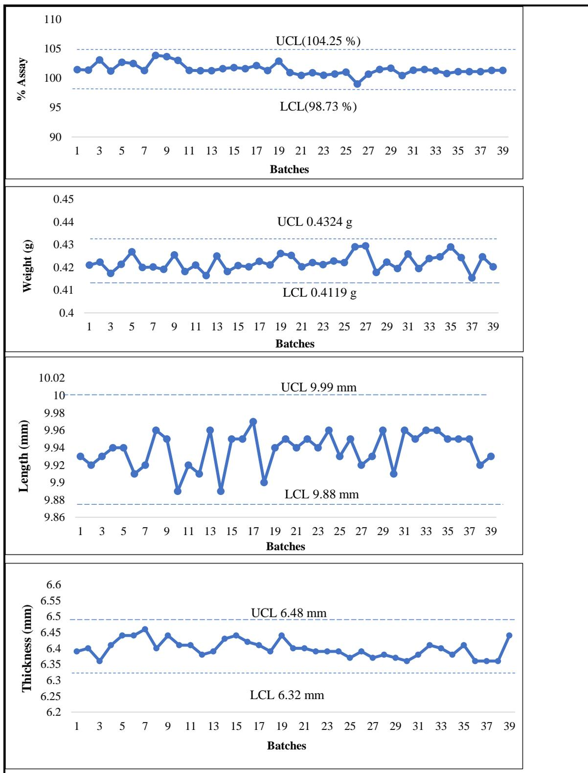
**Figure 2: X-bar charts for the assay, weight, length and thickness of ibuprofen coated tablets (n=39). UCL and LCL = upper control limit and lower control limit.**
