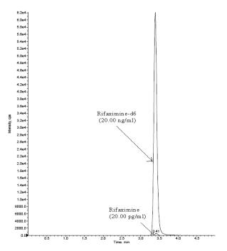
Figure 4: MRM chromatogram of Rifaximin and Rifaximin D6 in human plasma spiked with 20 pg/mL Rifaximin and 20.0 ng/mL Rifaximin - D6
