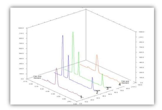
Figure 2: Typical densitograms pattern showing method specificity of solution containing folic acid reference standard and sample solution using a mobile phase containing ethyl acetate: methanol: ammonia (15:15:0.5 v/v), saturation time of 25 min using 10 cm x 10 cm HPTLC plate and 5  $\mu$ L application volume at a detection wavelength of 280 nm. Folic acid (0.125 mg/mL) R<sub>f</sub> 0.27 and 0.67. Track 1 and 4: Folic acid reference standard; Track 2 and 3: folic acid sample tablet.
