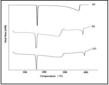
Figure 1: DSC of acetaminophen (a), acetaminophen granules prepared with Eudragit RL-100 (b) and Eudragit RS-PO (c).
