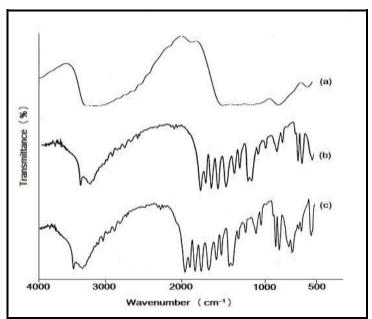
Figure 2: FTIR of acetaminophen (a), acetaminophen granules prepared with Eudragit RL-100 (b) and Eudragit RS-PO (c).
