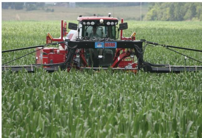
Fig. 2. Plant chlorophyll sensors used to adjust nitrogen fertilizer application.
