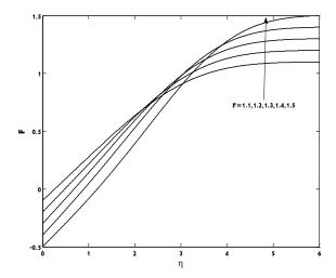
**Figure 4:** Velocity profile for some values of r in an interval [1.1, 1.5].
