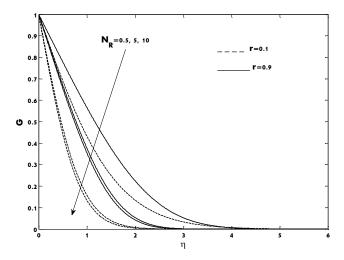
**Figure 7:** Effect of radiation parameter NR on temperature. When Pr=7
