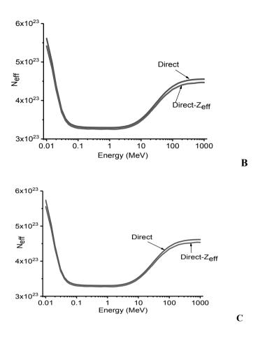
Figures 2 N<sub>eff</sub> as a function of energy for 5CB (A), 7CB (B), and 9CB liquid crystals
