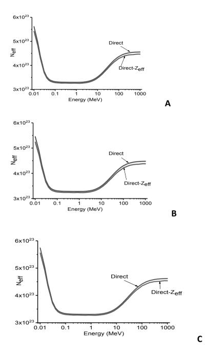
Figure 1.  $N_{\rm eff}$  as a function of energy for 5CB (A), 7CB (B), and 9CB (C) liquid crystal.
