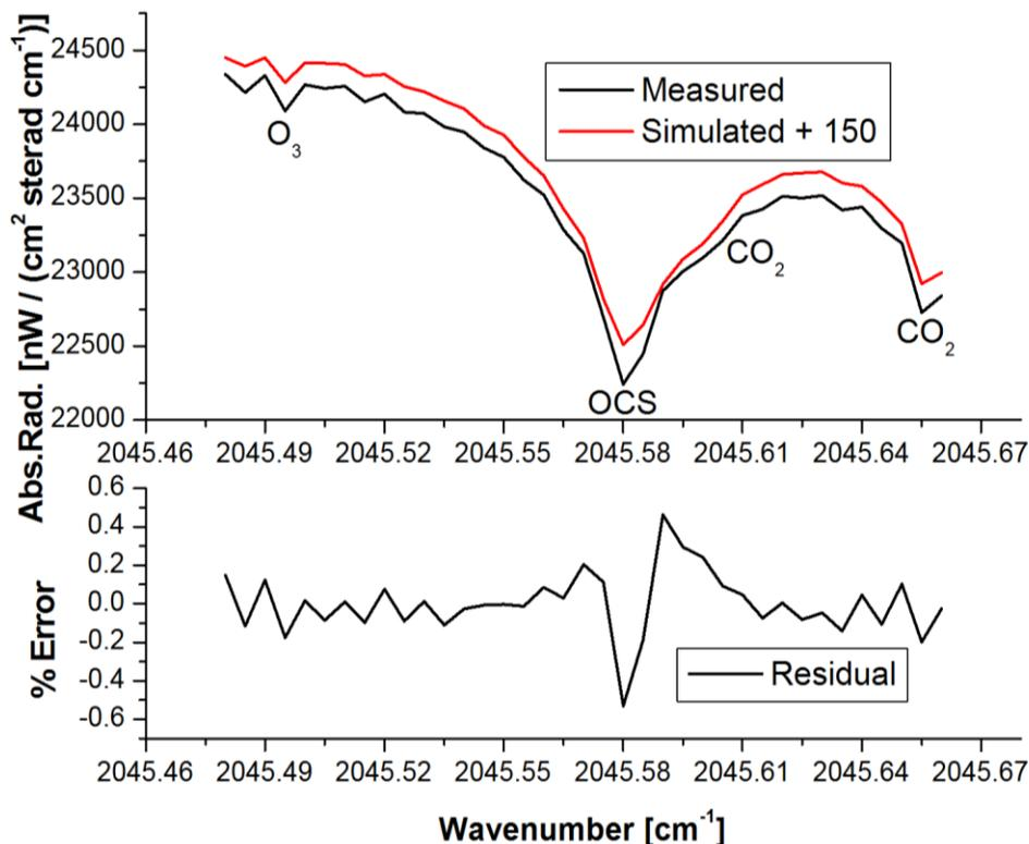
**Fig. 5.** Measured and calculated spectra
