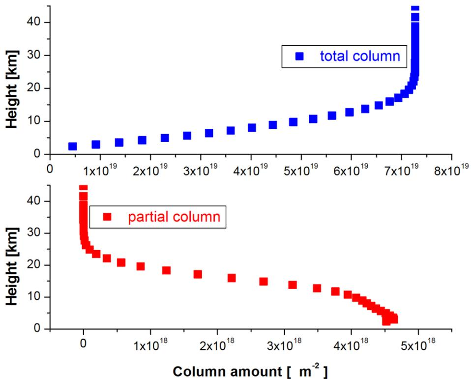
**Fig. 8.** Partial and integrated columns of OCS on the 27 January 2010.
