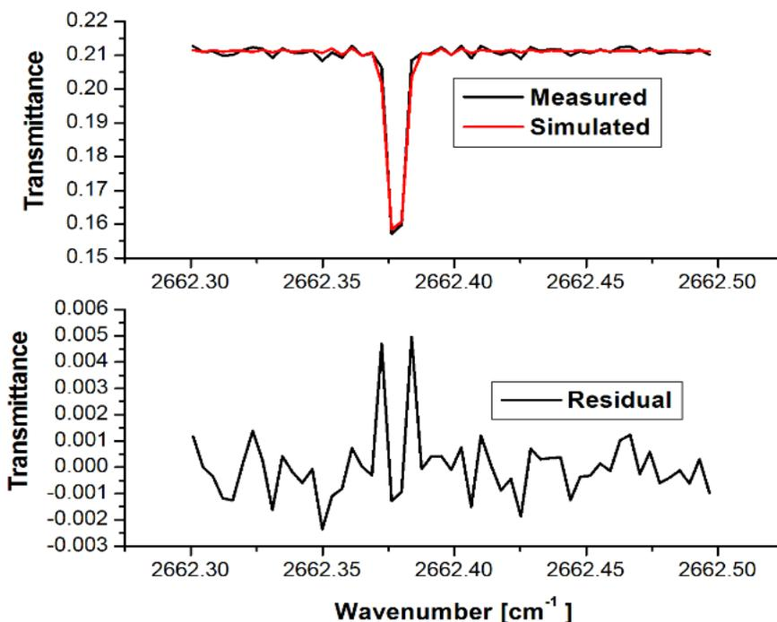
**Fig. 1.** The measured and simulated spectral fit with the corresponding residual spectra for the date of 01 June 2009.
