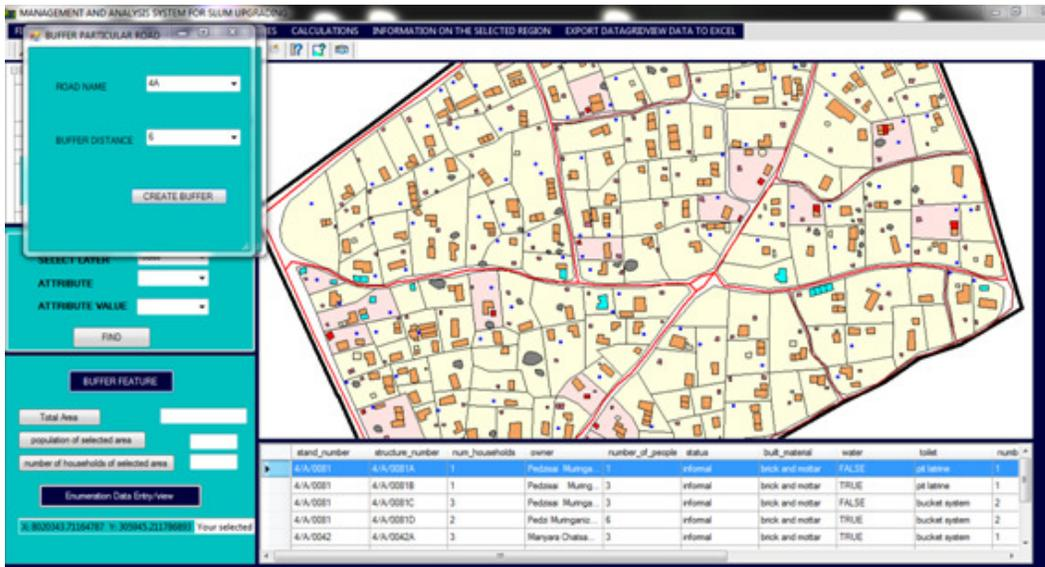
Figure 7: Shows selected structures that are within 6m from road 4A
