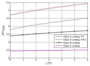
Figure 4: Power consumption of 2X2, 3 sector MIMO BTS as a function of climate factor ( $\chi$ ) and the AC cooling class.
