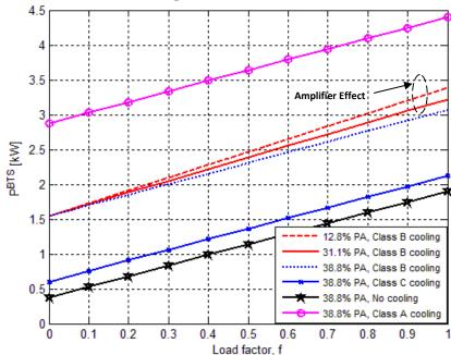
Figure 2: Power consumption of base station as a function of power amplifier efficiency and air conditioning
