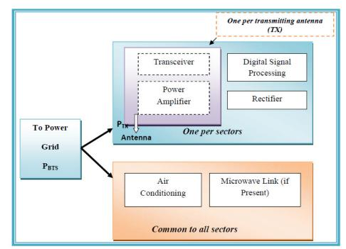
Figure 1: Block diagram of base transceiver station (BTS)
