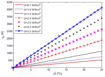
Figure 3: Heat Flux as a function of change in ambient and outside temperatures and Thermal transmittance.
