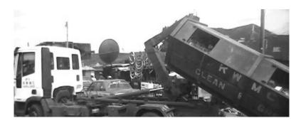
Plate 1: Dyno Truck lifting a Ro-Ro bin.
