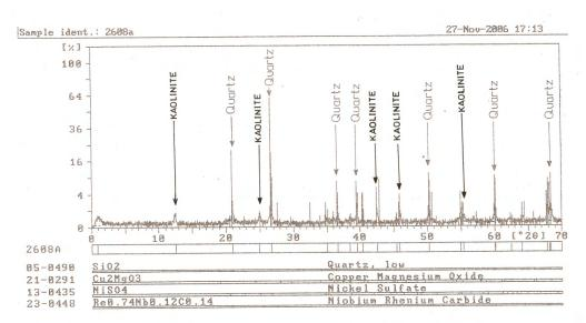
Fig. 2. X -ray diffraction result of Kutigi clay Loc A1/ sample 1.
