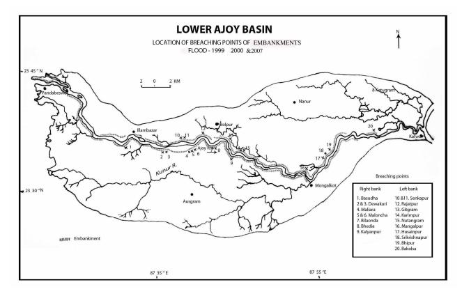
Figure 3 Breaching Points of Embankments
