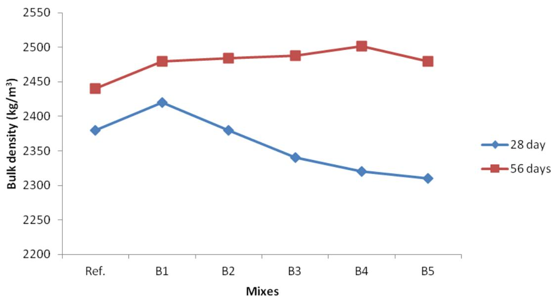
Figure 6 Variation between bulk density and mineral composition for Set B
