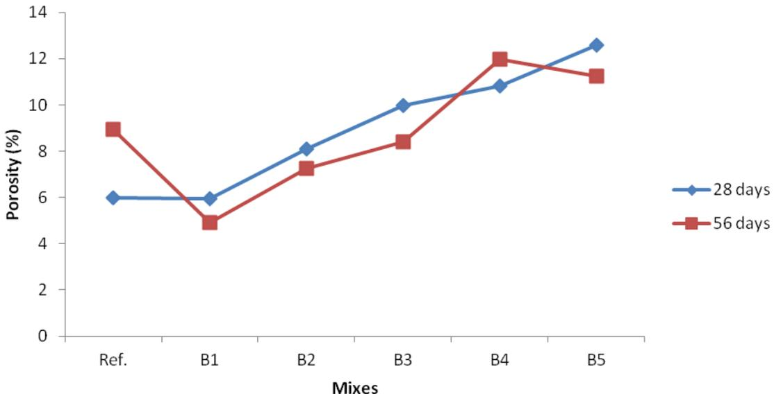
Figure 4 Porosity value for Set B mixes at 28 and 56 days hydration
