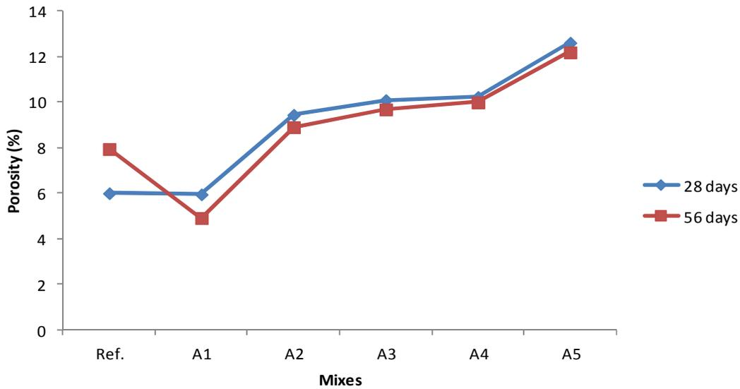
Figure 3 Porosity value for Set A mixes at 28 and 56 days hydration
