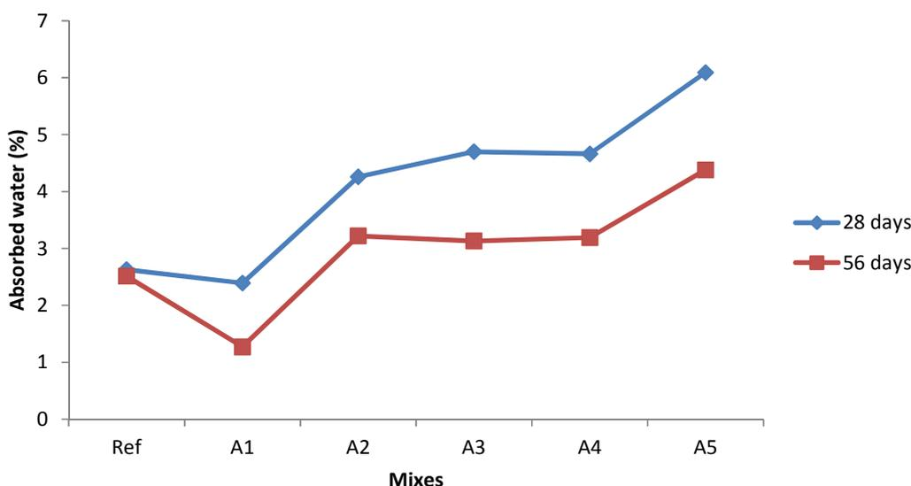
Figure 1 Water absorption for Set A mixes at 28 and 56 days hydration
