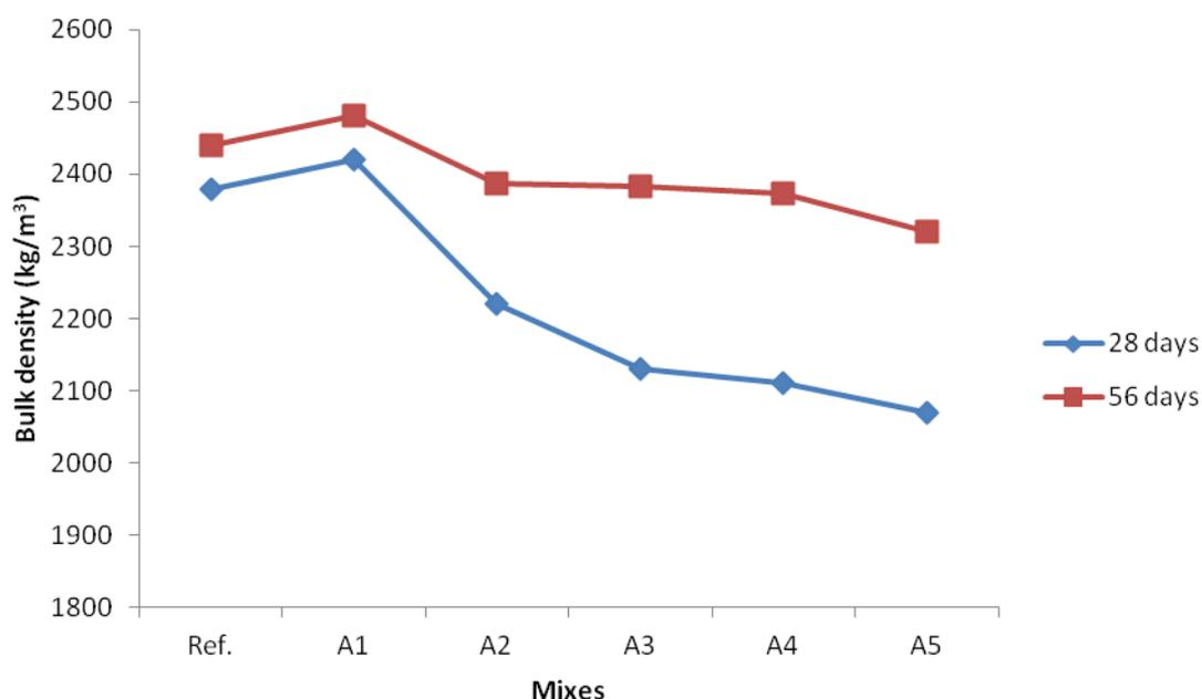
Figure 5 Variation between bulk density and mineral composition for Set A
