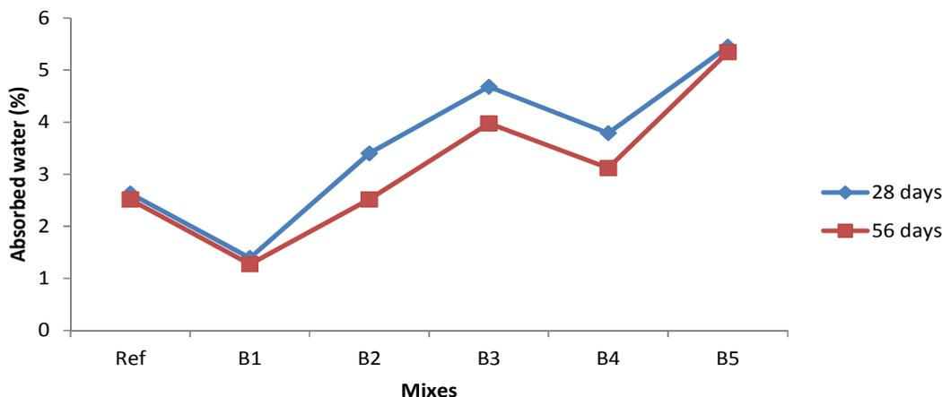
Figure 2 Water absorption for Set B mixes at 28 and 56 days hydration
