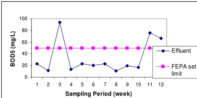
Figure 1 A trend plot of BOD<sub>5</sub> compared with FEPA set limit
