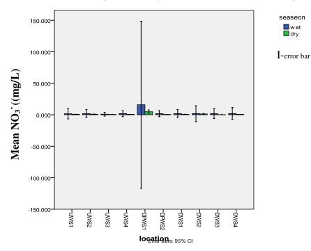
Figure 6: Mean seasonal variation in the nitrate ion concentration of the water samples Key: Uws – Upstream water sample, Dpws- Discharge point water sample, Dws- Downsteam Water Sample
