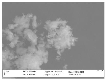
Figure 2: Maize cob char SEM image
