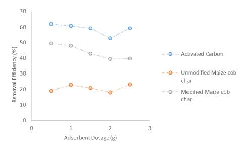
Figure 5: Effect of dose of the adsorbents on the removal efficiency of Cr (VI). Cr (VI) Concentration: 30 mg/L; Agitation time: 60 min; Agitation speed 400 osc/min
