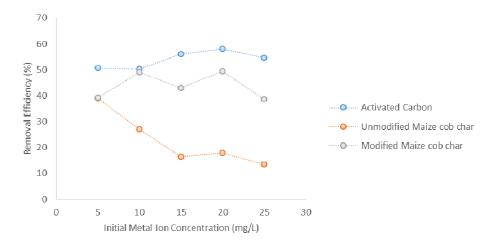
Figure 3: Effect of initial ion concentration on removal efficiency of Cr (VI) by the adsorbents. Agitation time: 45 min; agitation speed: 400 osc/min; dose of each adsorbent: 1.5 g.
