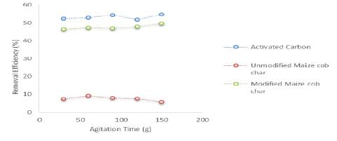
Figure 7: Effect of agitation time on removal efficiency of Cr (VI) by the adsorbents. Cr (VI) Concentration: 20 mg/L; agitation speed: 400 osc/mim; dose of each adsorbent: 1.0 g
