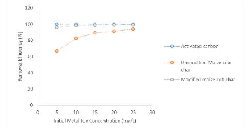
Figure 4: Effect of initial ion concentration on removal efficiency of Pb (II) by the adsorbents. Agitation time: 45 min; agitation speed: 400 osc/min; dose of each adsorbent: 1.5 g.
