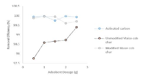
Figure 6: Effect of dose of the adsorbents on the removal efficiency of Pb (II). Pb (II) Concentration: 30 mg/L; Agitation time: 60 min; Agitation speed 400 osc/min
