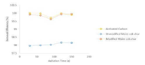
Figure 8: Effect of agitation time on removal efficiency of Pb (II) by the adsorbents. Pb (II) Concentration: 20 mg/L; agitation speed: 400 osc/min; dose of each adsorbent: 1.0 g
