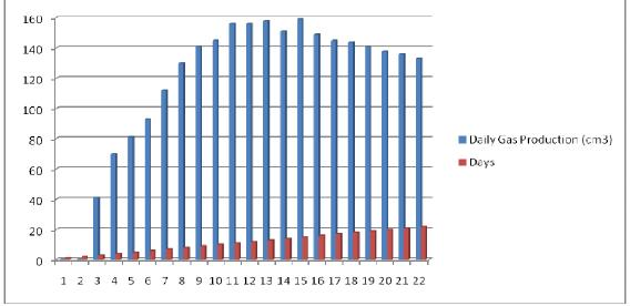
Figure 3: Gas produced for a restarted digester
