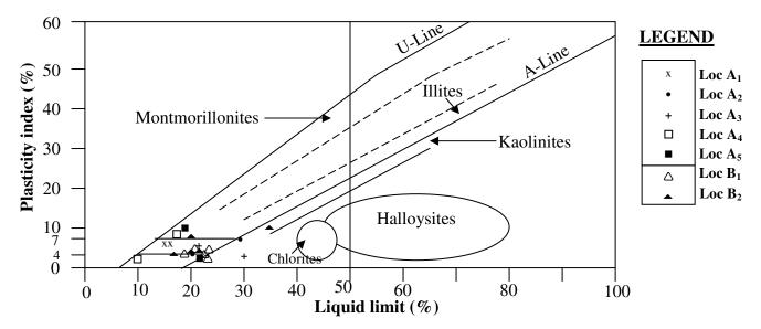
**Fig.3**: Modified plasticity classification chart plotted for Kutigi clay (after USBR 1963)
