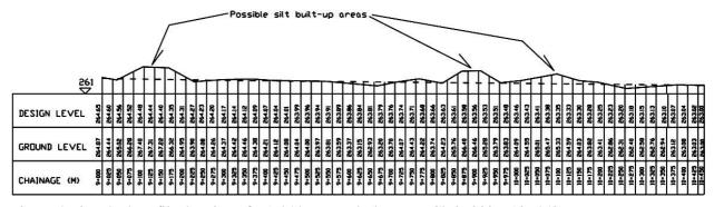
Figure 4 River bed profile drawing of a 1.45 km stretch (between Ch 9+000 - 10+450)
