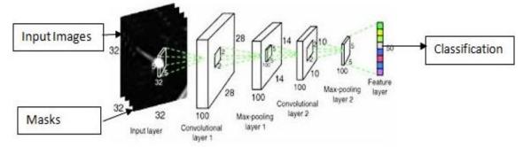
Figure 3: Proposed architecture of convolutional neural network
