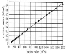
Fig. 6: Curve of shear stress vs particle radius  $\tau = 0.0005r_n$ , R<sup>2</sup>=0.9982.
