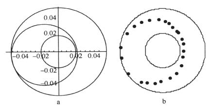
**Fig. 5:** Comparison of the trajectory of a microcarrier particle by model simulation results (a) and experiment data (b). (r=1308 kg/m<sup>3</sup>, r<sub>p</sub>=730  $\mu$ m, .  $\omega_p = \omega_i = -40$  rpm).
