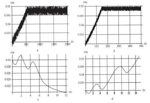
**Fig. 4:** Radial position of the particle vs the time  $(r_p=100 \ \mu.m)$ . a: $\omega_0 = \omega_i = 15$ rpm; b:  $\omega_0 = \omega_i = 30$ rpm; c:  $\omega_0 = 30$ rpm; d: .  $\omega_0 = 10$ rpm; d: .  $\omega_0 = 10$ rpm;  $\omega_i = 30$ rpm.
