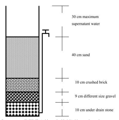
Fig.1 Components of MHMF<sub>2</sub> (with crushed brick). Note to the scale
