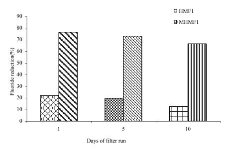
Fig.2 Effect of crushed brick on fluoride reduction
