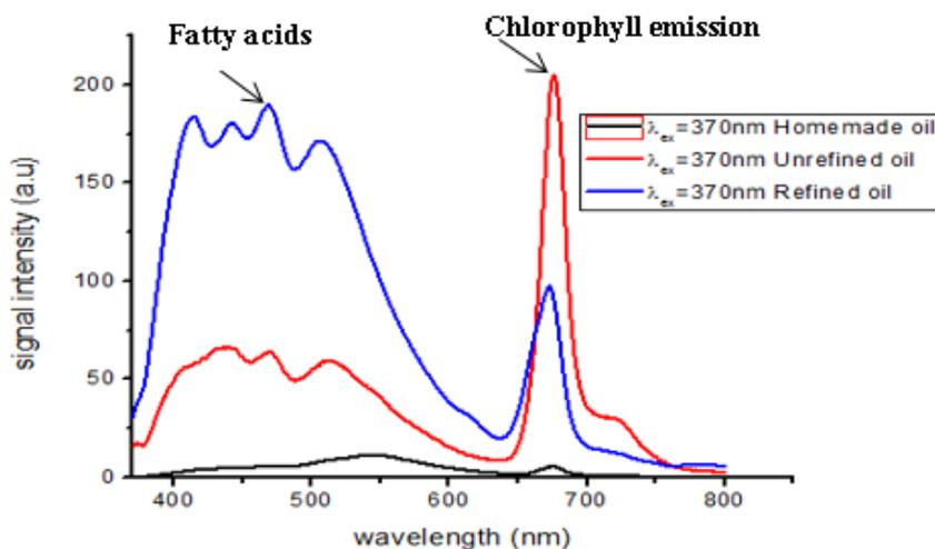
**Figure 4.** Comparison of Spectral Peaks for Home-Made, Unrefined and Refined Niger Seed Oils of Different Acidity (pH)
