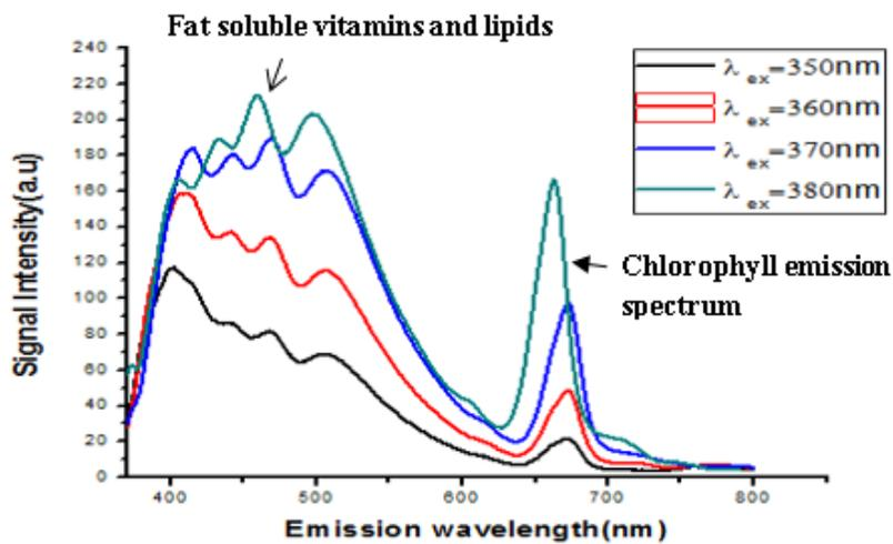
Figure 3: Fluorescence Intensity versus Wavelength of Refined Niger Seed Oil
