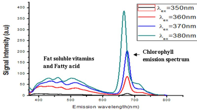
Figure 2: Fluorescence Intensity versus Wavelength of Unrefined Niger Seed Oil
