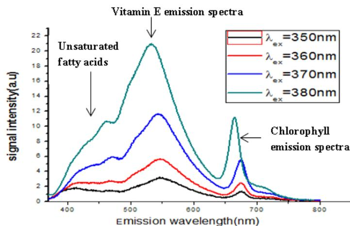
**Figure 1:** Fluorescence Intensity versus Wavelength of Homemade Niger Seed Oil
