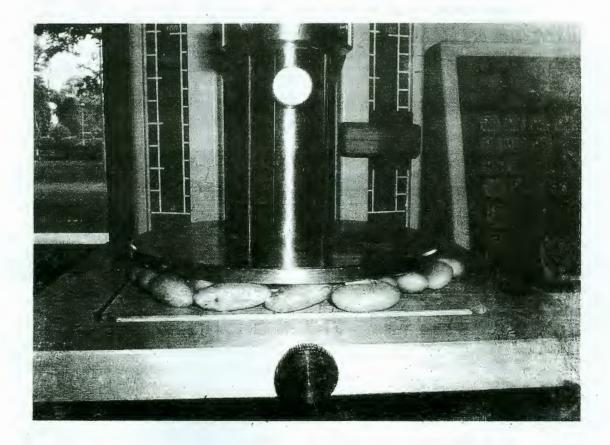
Figure 1: Texture analyzer (Model LRX 5K, TA 500, LLOYD Instruments, England,
